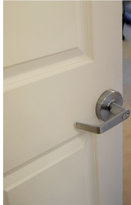
This lever for standard locks meets ADA requirements for "no grasping, twisting, or pinching movements" to operate the opening. It can easily be operated, even with an elbow.
