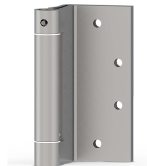
This swing-clear hinge features 90-degree bend that holds the door completely away from the frame when in the open position. This feature provides more space in a narrow frame to reach the 32" clear width required by ADA.
